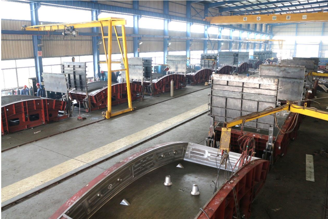
Assembly production Line for OD13.5M segment mould.
