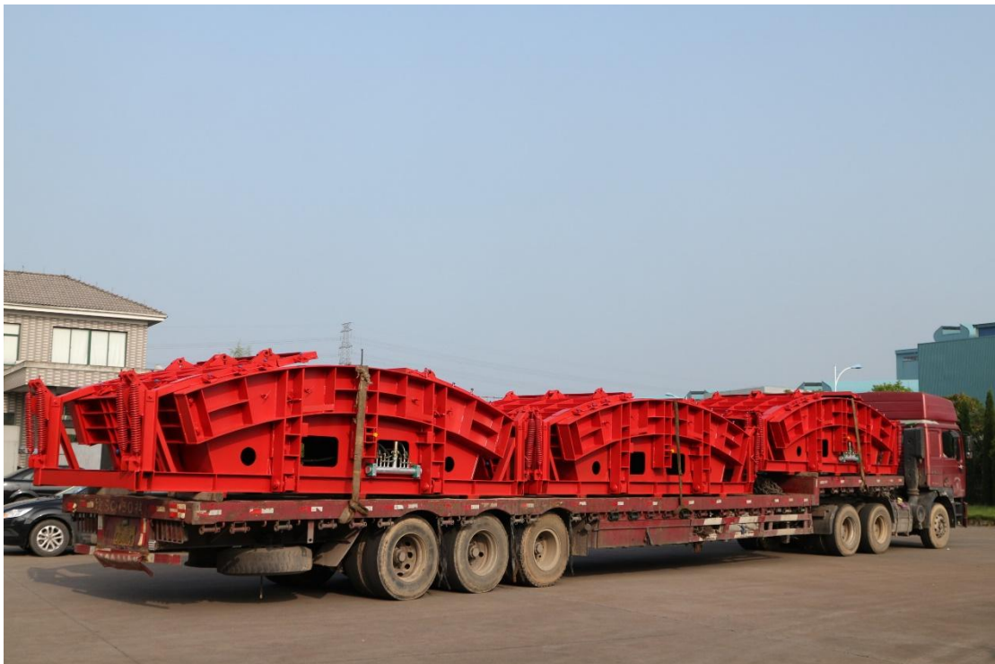
Delivery of OD 13.5M segment mould for Hong Kong- TMCLK project's precast yard.
